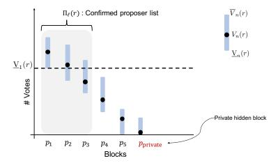
Fig. 13: In the above example, public proposer block  $p_1$  has the largest lower confidence bound, which is larger than the upper confidence bound of the private block. So list confirmation is possible and the list confirmed is  $\Pi_{\ell}(r) = \{p_1, p_2, p_3\}$ .
