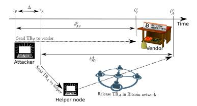
Figure 4: Sketch of a double-spending attack on fast payments in Bitcoin. Here, the attacker  $\mathcal{A}$  dispatches two transactions that use the same BTCs in the Bitcoin network. The double-spending attack is successful if the BTCs that  $\mathcal{A}$  used to pay for  $\mathcal{V}$  cannot be redeemed (i.e., when the second transaction is included in the upcoming Bitcoin block).
