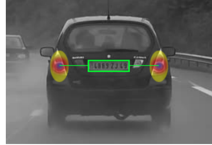
Fig. 4. Mapping of \phi (license plate location) to T\{\phi\} (light modulation source) for a car. A gaussian kernel is used at the location of T\{\phi\} to weight the pixels close to the light modulation source, which reduces errors due to relative movements of the vehicles and distortions on the mapping of T\{\phi\} and normalisation is applied to allow the relaxation of dependence of the distance between vehicles.
